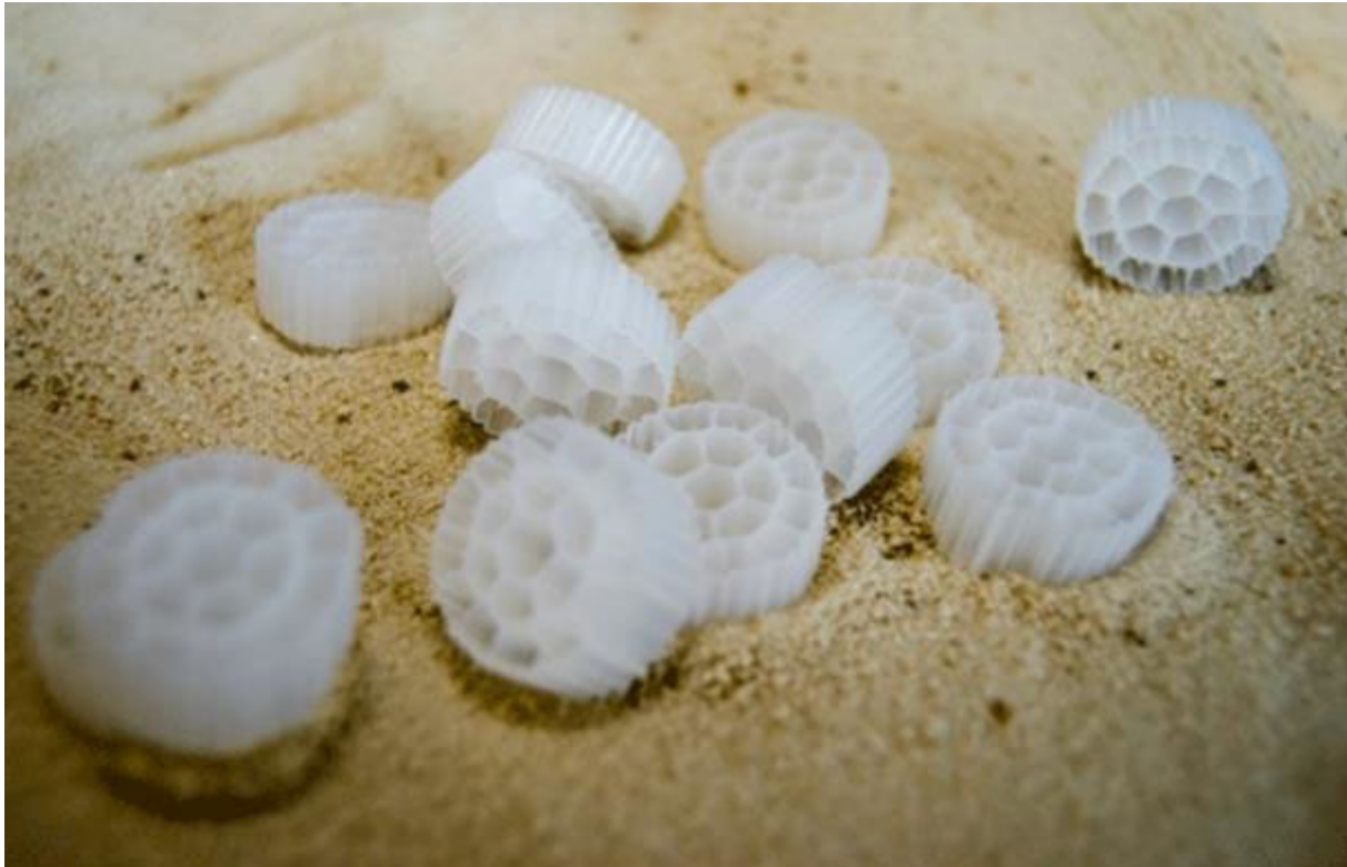
Figure 1. Plastic carriers for location of bacteria to accumulate P from waste water, placed on top of crystals of struvite (magnesium-ammonium phosphate) precipitated from waste water at the Hias IKS waste-water treatment plant, Hedmark, Norway. Photo: VA-Nytt (forskning.no)
